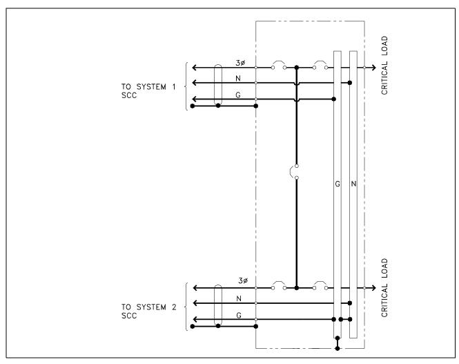
Multi-Module Systems can be used with Power-Tie switchgear to provide dual critical load busses. The Power-Tie switchgear permits transferring critical loads from one critical bus to the other so that one UPS system and associated breakers can be de-energized for maintenance. Certain configurations of Power-Tie equipment also permit the operator to continuously parallel the output of both UPS systems.
